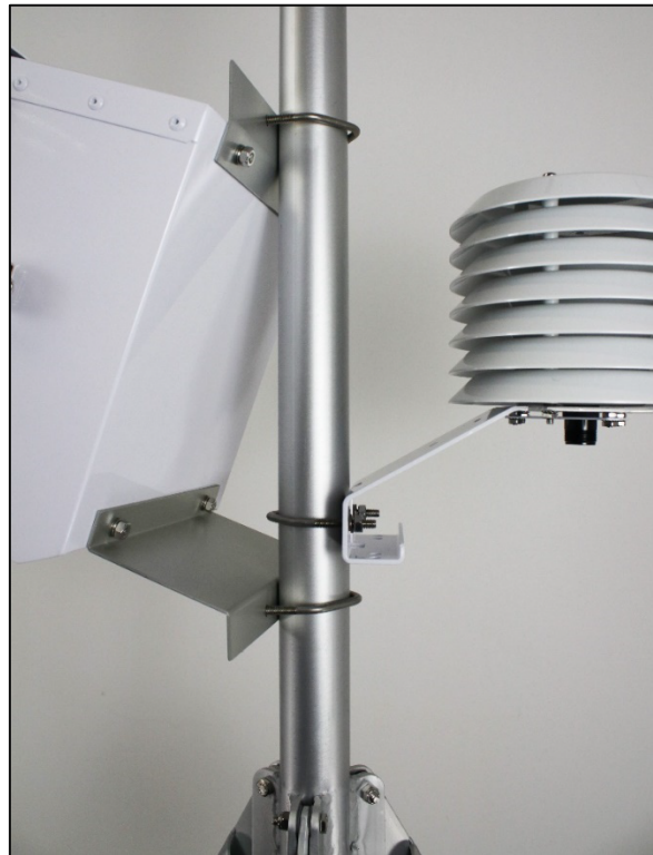
Figure 4-16 Control Unit Mounting Detail
