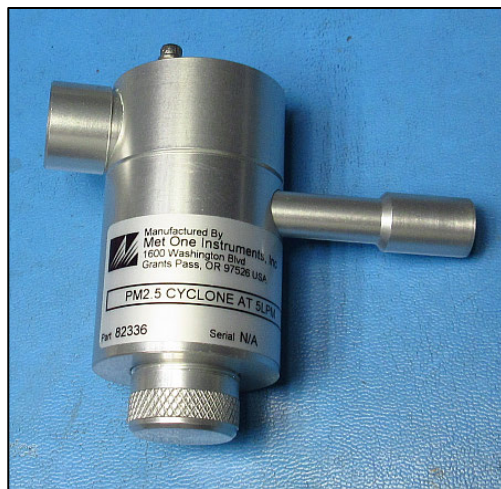
Figure 6-4 Unscrew and Clean Particle Trap
