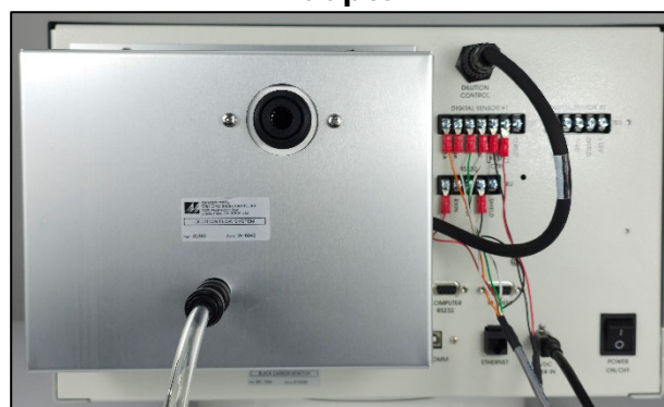
Figure 2-10 Dilution Flow System Installed
