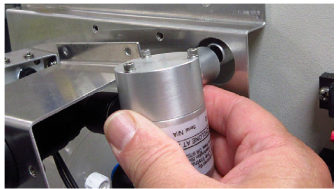
Figure 6-9 Pull Cyclone Away from BC 1054 Inlet Fitting
