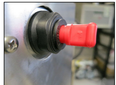
Figure 6-16 Leak Check Sealing Plug Installation
