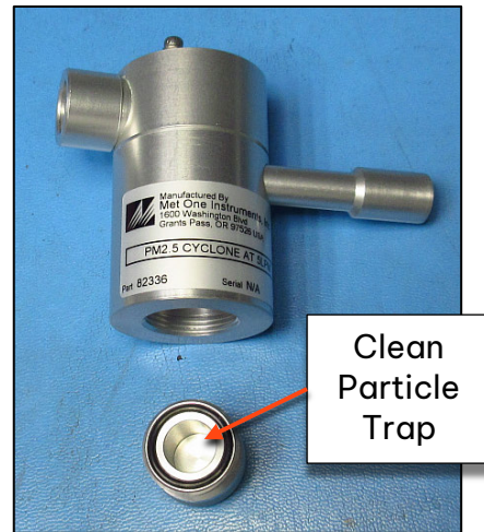
Figure 6-4 Unscrew and Clean Particle Trap
