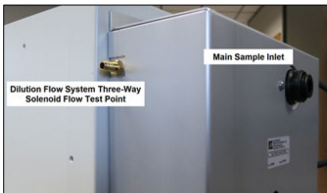
Figure 6-26 Dilution Flow Test Point
