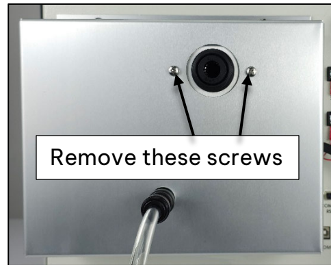
Figure 2-6 Dilution Flow System Cover Removal
