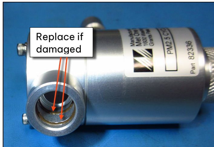
Figure 6-7 Cyclong Inlet O-rings
