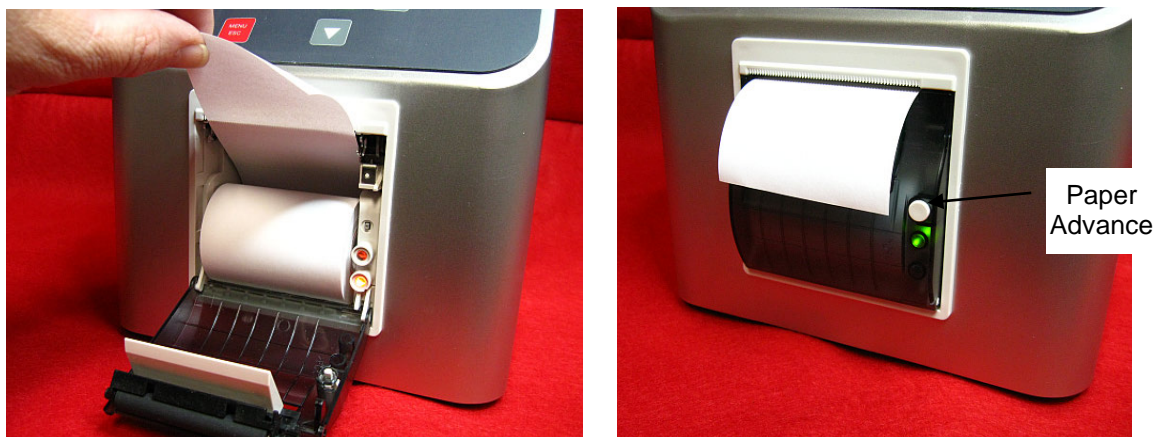
Figure 6 – Install Paper and Close Printer Door
