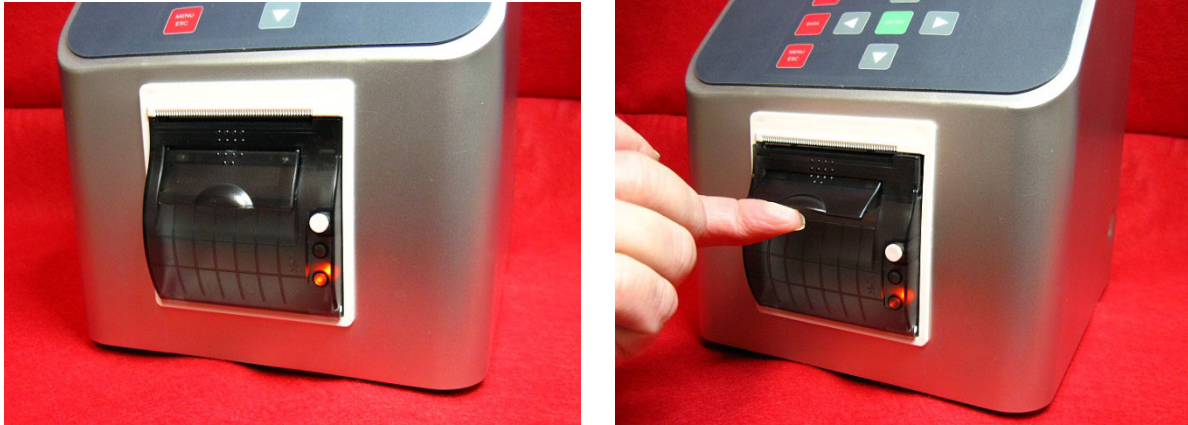
Figure 5 – Open Printer Door
