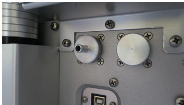
Figure 6-4 Sheath Air Inlet Covered
