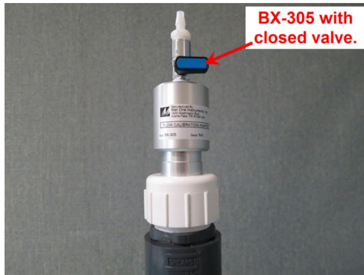
Figure 6-2 BX-305 Installed on Inlet Tube
