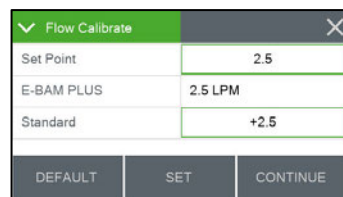
Figure 6-13 Sheath Air Calibration Screens
