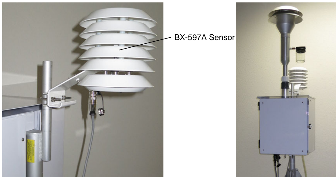
Figure 2-3 Mounting the BX-597A Sensor
