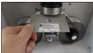
Figure 6-18 Starting the Span Test
