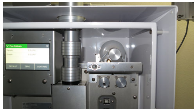
Figure 6-3 Flow System Cover Removed
