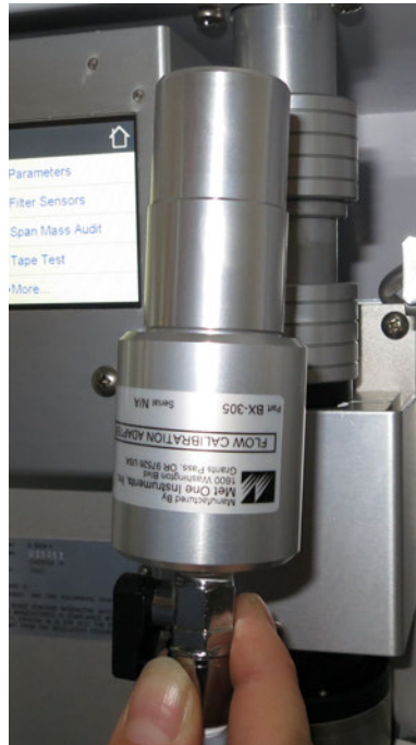
Figure 6-12 Connecting the CTS to the Sheath Air Pre-Filter Inlet
