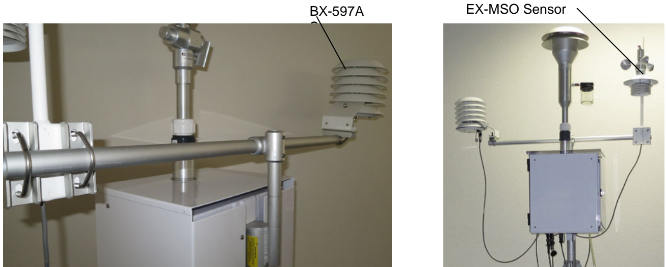
Figure 2-4 Sensor Mounting with an Optional Wind Sensor
