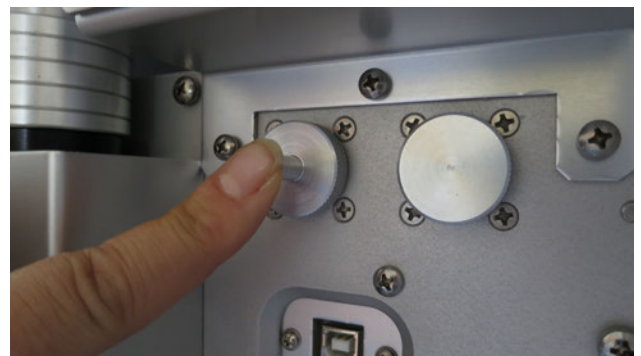
Figure 6-4 Sheath Air Inlet Covered
