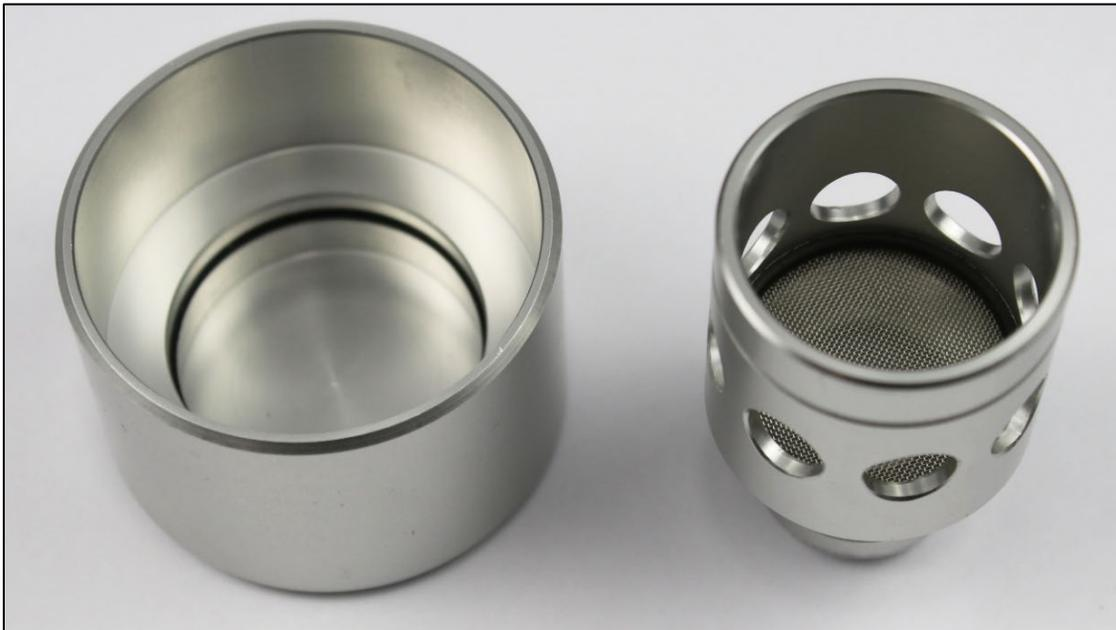
**Figure 6-2 Inlet Assembly**
