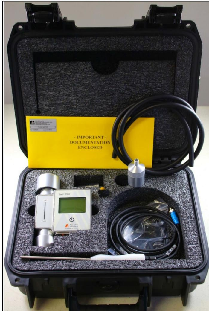
**Figure 2-1 Standard Components for the Swift 25.0**
