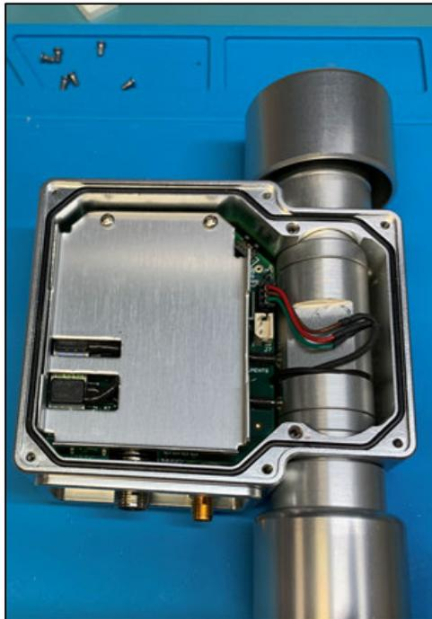
Figure 6-5 Battery Tray Removal
