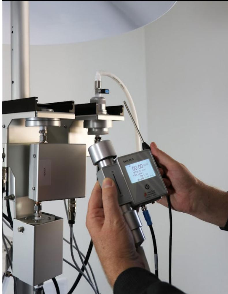
**Figure 4-2 Connection to a SASS with Tubing Adaptors**
