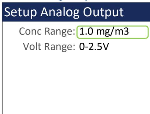
The screenshot shows a screen titled "Setup Analog Output" with a dark blue header. Below the header, there are two rows of text: "Conc Range: 1.0 mg/m3" (with "1.0 mg/m3" in a green-bordered input field) and "Volt Range: 0-2.5V".
