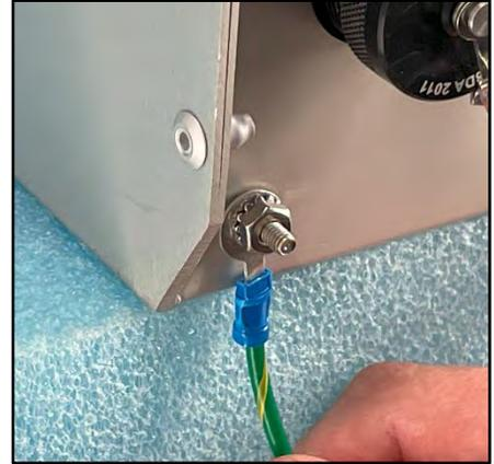
**Figure 2-2 Grounding Wire Installed and Secured**
