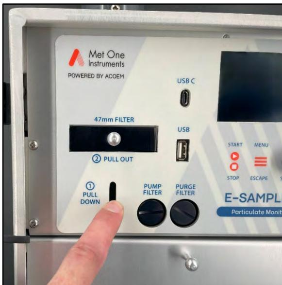
**Figure 8-5 Filter Cassette Holder Removal**
