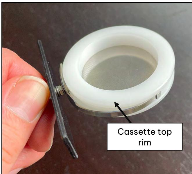
**Figure 8-7 47 mm Filter Holder, Top View**
