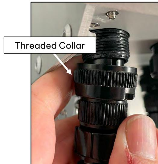
Figure 4-19 Connector Alignment and Threaded Collar
