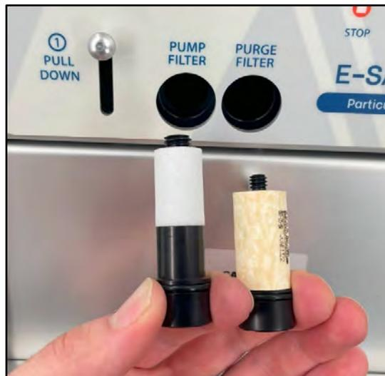
**Figure 8-20 Pump and Purge Filters Removed**
