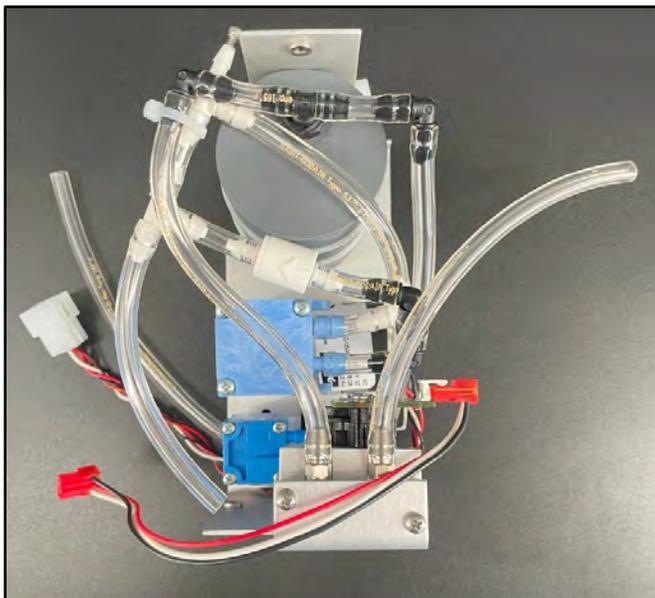
**Figure 8-21 Pump Module Top View**
