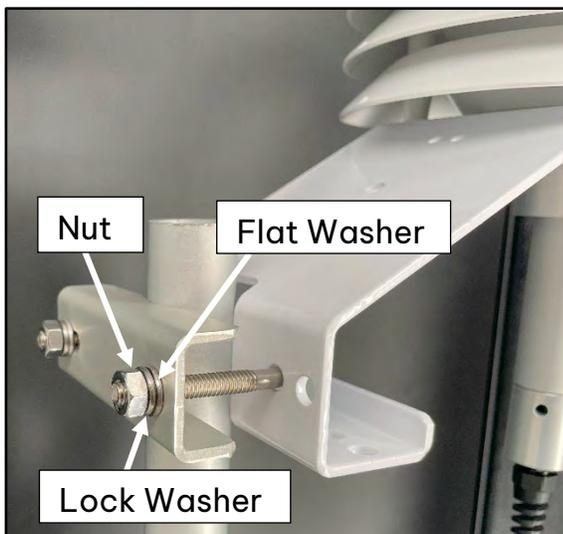
**Figure 4-15 Sensor Mounting Example 1**
