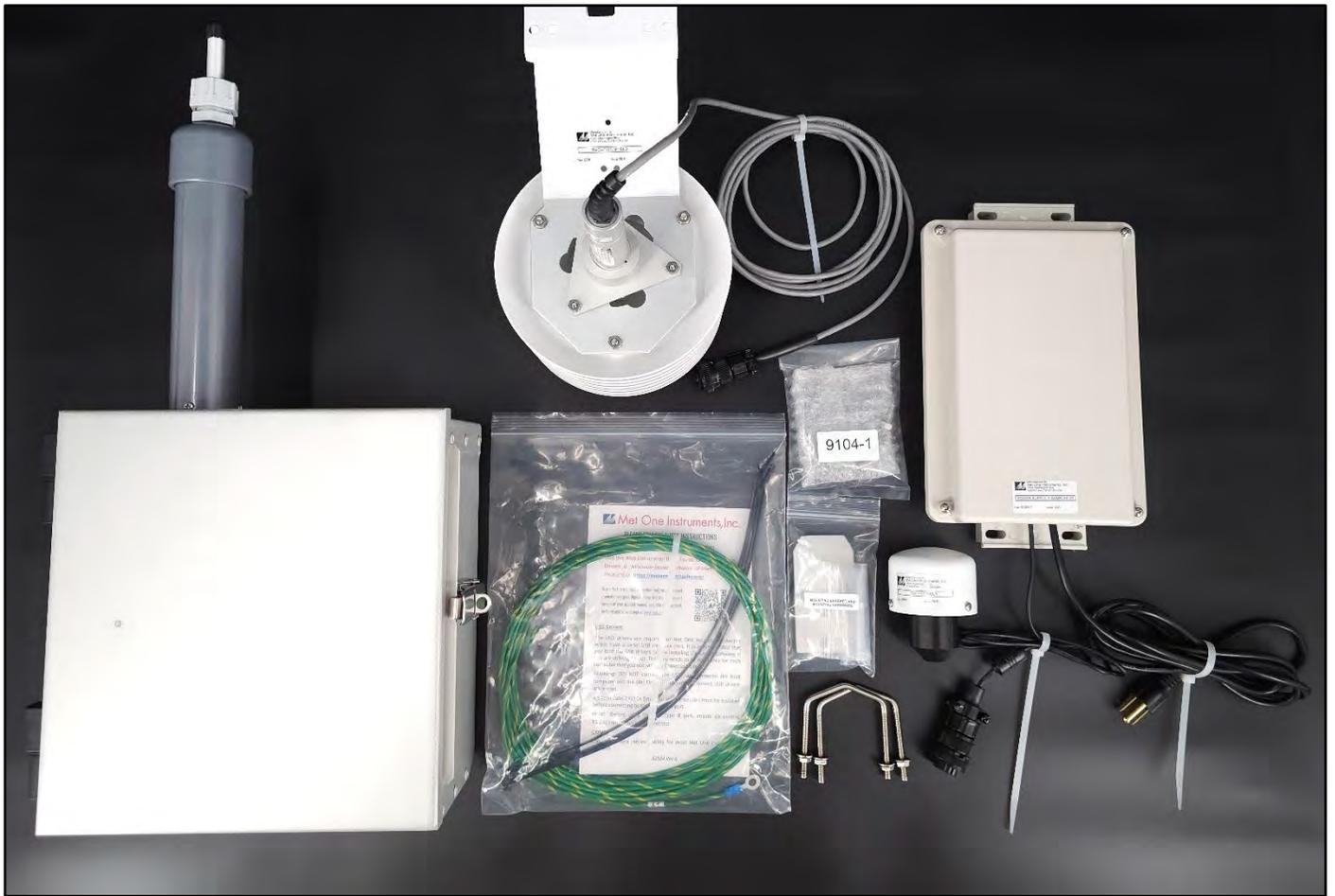
**Figure 3-1 E-Sampler V2 Standard Accessories**
