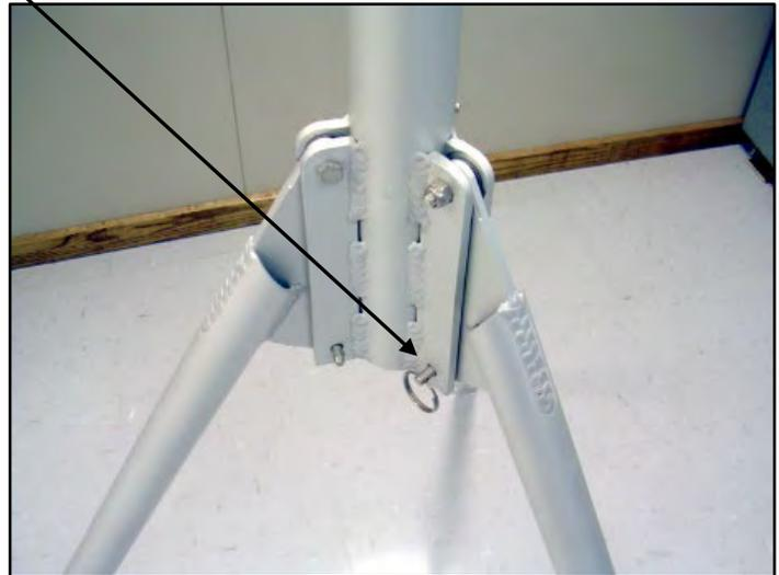
**Figure 4-5 Tripod Legs Deployed**
