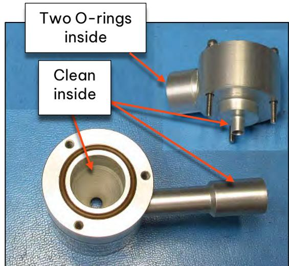
**Figure 8-3 Cyclone Internal Cleaning**
