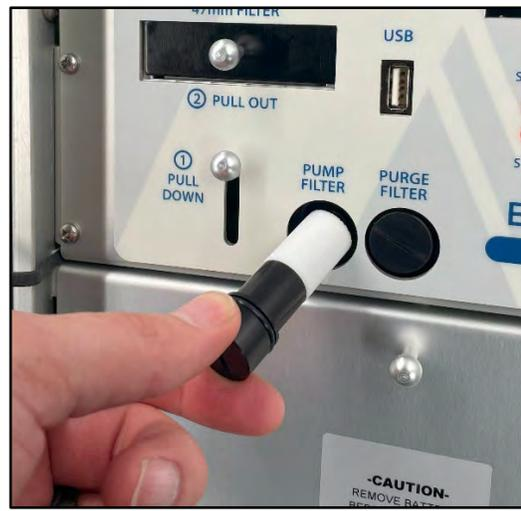
**Figure 8-19 Removing Filter and holder**
