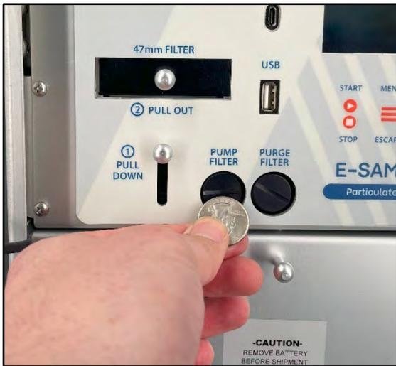
**Figure 8-18 Unscrewing Filter Holder**
