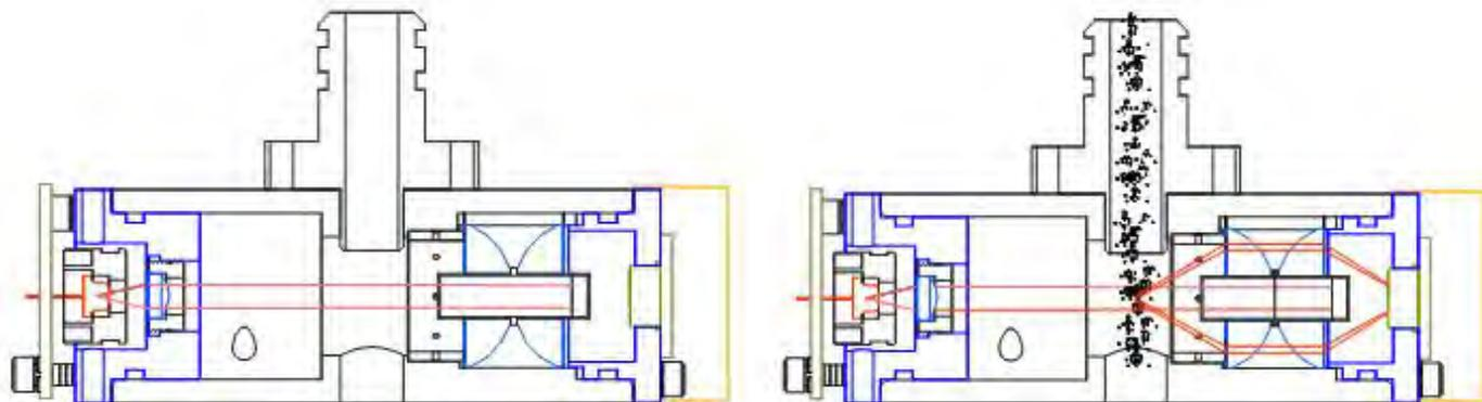
**Figure 11-2 Clean Air and Particulate Scatter Conditions In the MD-F Engine**
