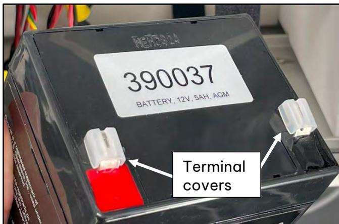
**Figure 4-28 Battery Terminal Covers**
