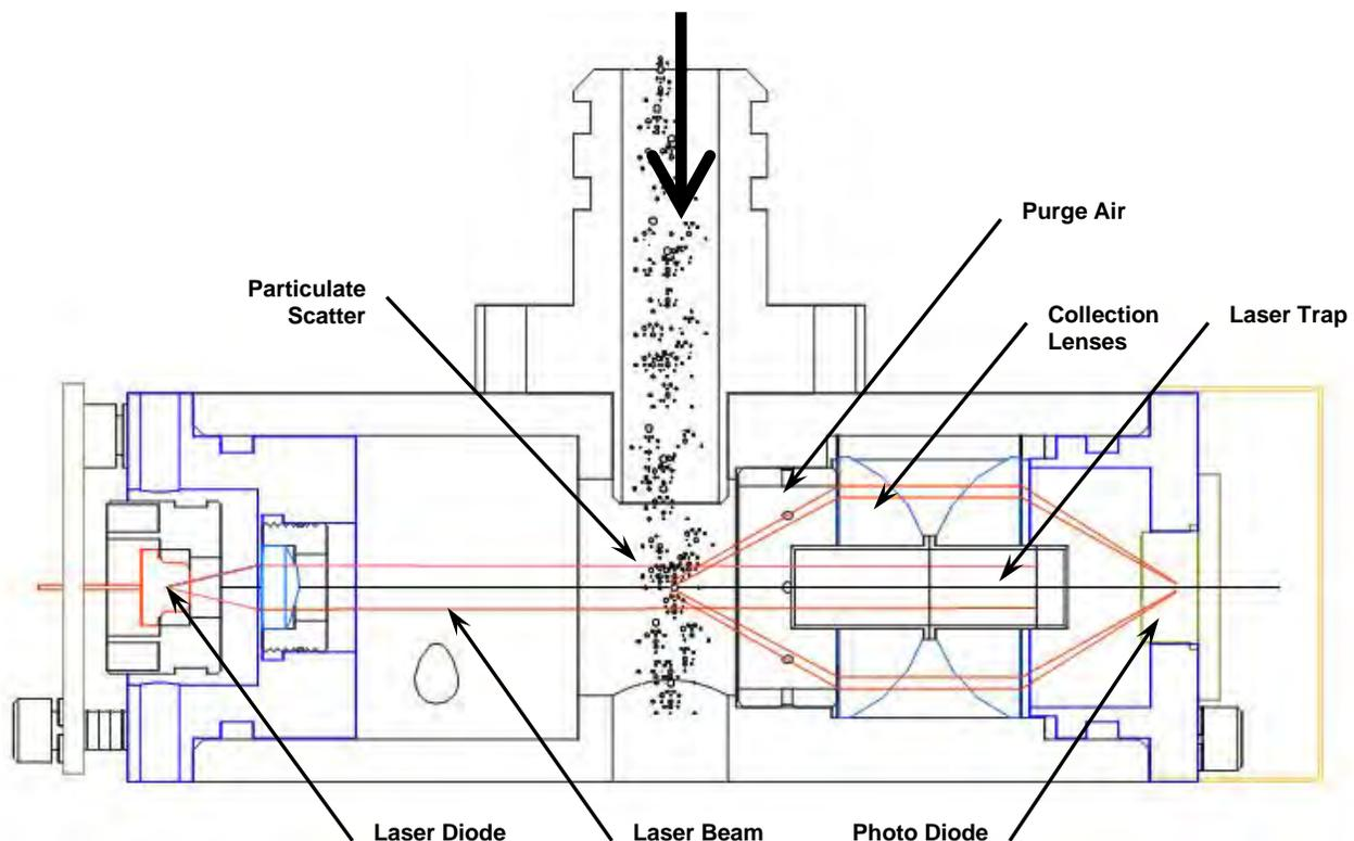
**Figure 11-1 MD Forward Light Scatter Laser Optical Engine**
