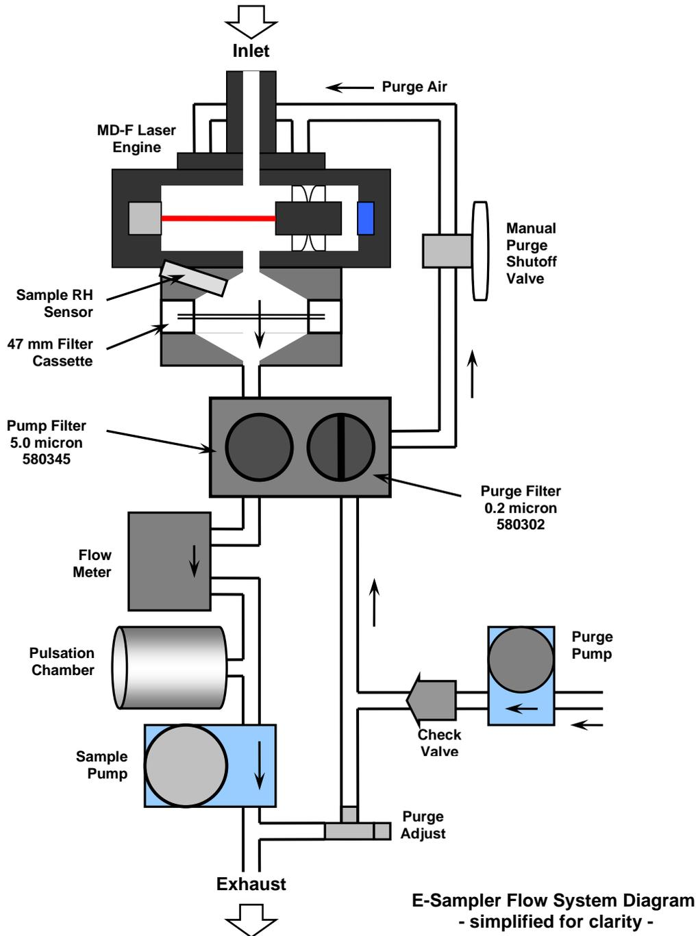
**Figure 11-4 E-Sampler V2 Flow System Diagram**
