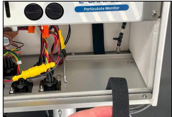
**Figure 4-27 Battery Retention Strap**
