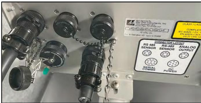
**Figure 4-24 DC Power Connected**
