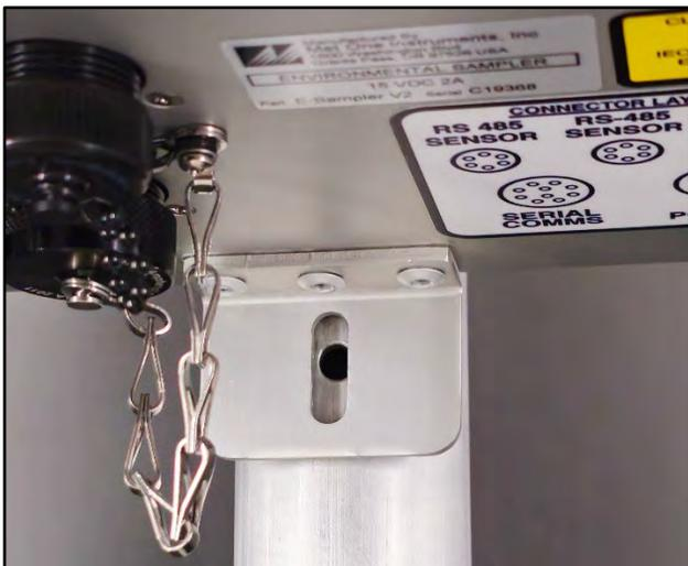
**Figure 4-2 Bottom Mounting Support Tab**
