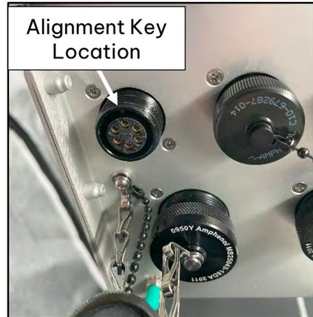
Figure 4-17 Sensor Plug alignment key
