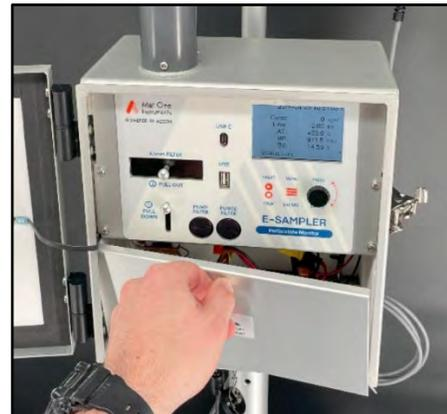
**Figure 4-25 Electrical Cover Removal**
