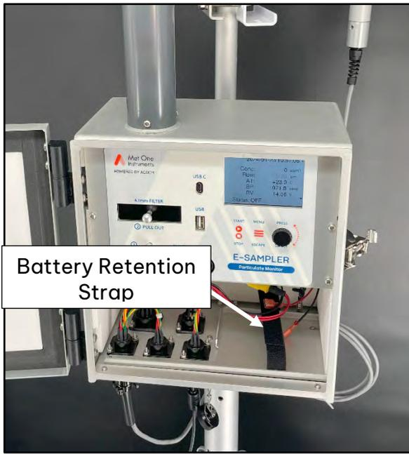
**Figure 4-26 Electrical Cover Removed**
