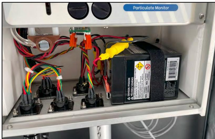
**Figure 4-31 Battery Installed**
