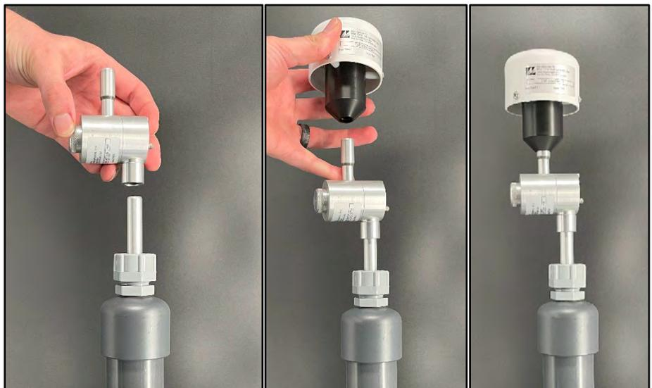
Figure 4-12 Inlet with TSP and Cyclone
