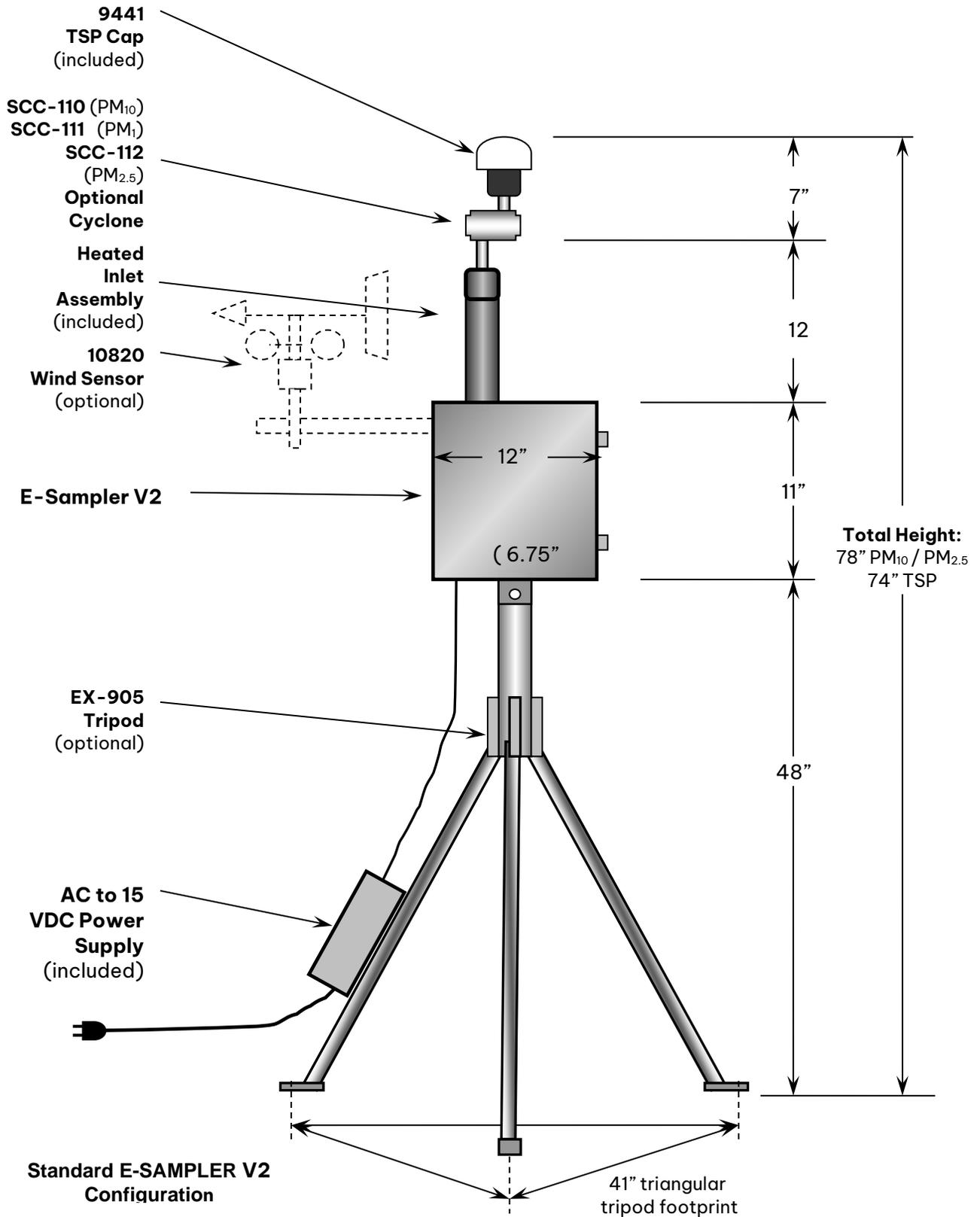
**Figure 1-2 E-Sampler V2 Full System Diagram**
