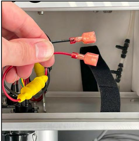
**Figure 4-29 Batter Connection Wires**
