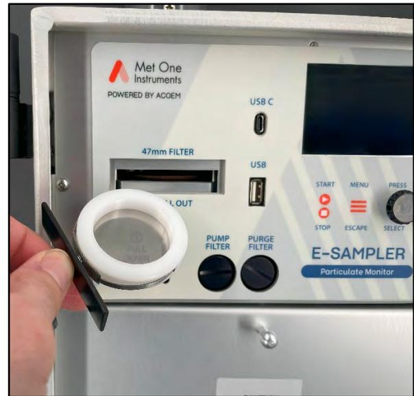
**Figure 8-6 Filter Cassette Holder Removed**
