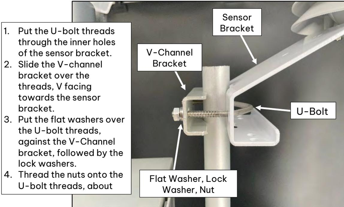
**Figure 4-14 Sensor Mounting Diagram**
