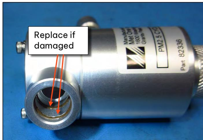
**Figure 8-4 Cyclone Inlet Receiver O-rings**
