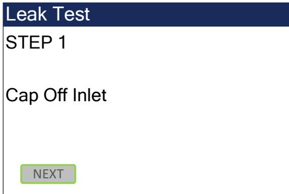
The Leak Test screen is used to check the flow system for leaks that can affect performance and accuracy. See **Section 8.3.1** for the leak test procedures.
