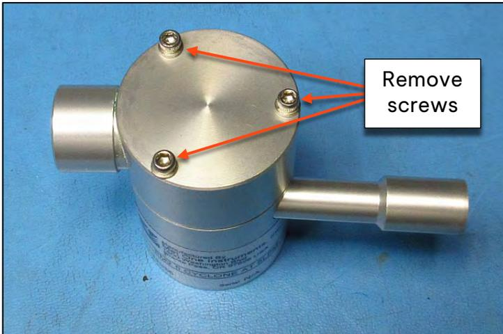
**Figure 8-2 Cyclone Disassembly for Full Cleaning**
