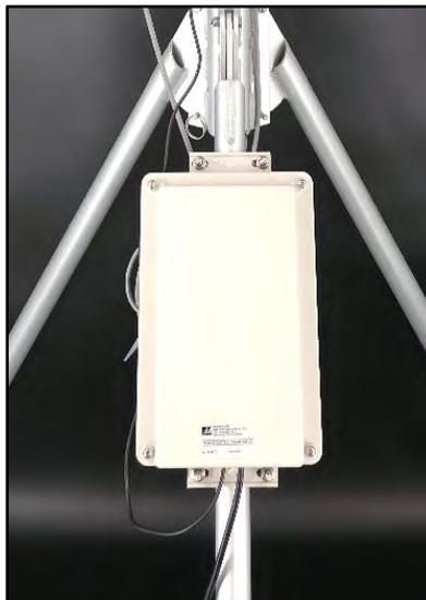
**Figure 4-22 Power Supply Mounted**
