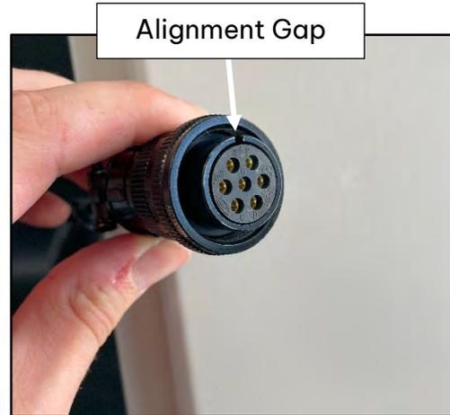
**Figure 4-23 Power Supply 7-Pin Connector**
