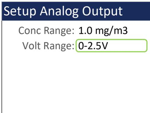
**Figure 6-22 Setup Analog Output, Volt Range Config.**
