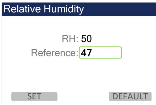
Figure 5-17 Calibrate Relative Humidity Screen
