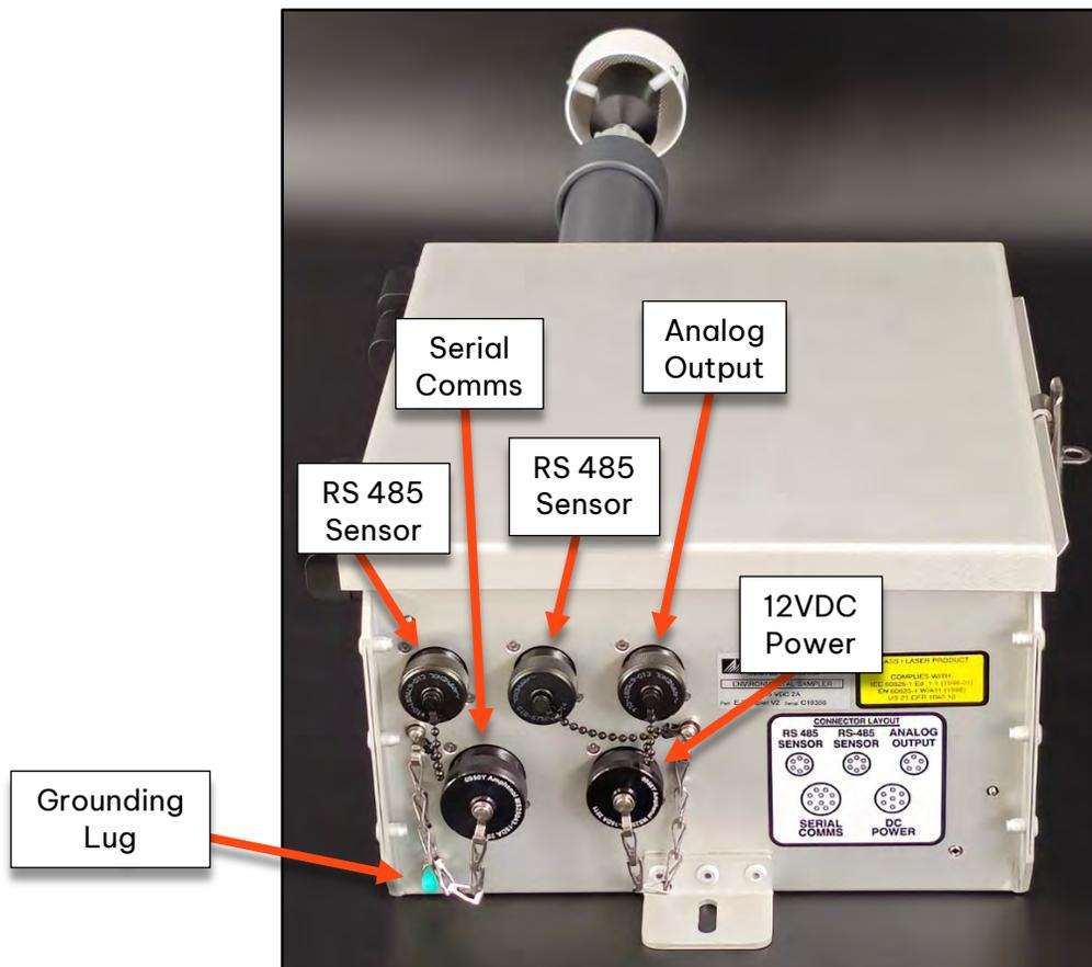
**Figure 4-13 Electrical Connections**
