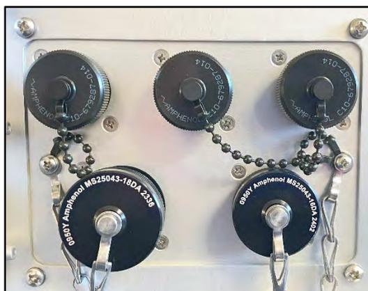
**Figure 8-23 Connector Plate Example**
