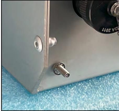
**Figure 2-1 Grounding Stud Cap and Nut Removed**
