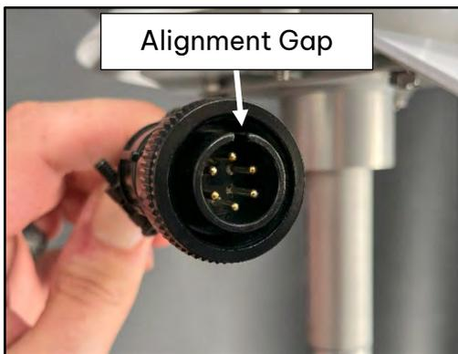
Figure 4-18 Sensor Connector Alignment Gap
