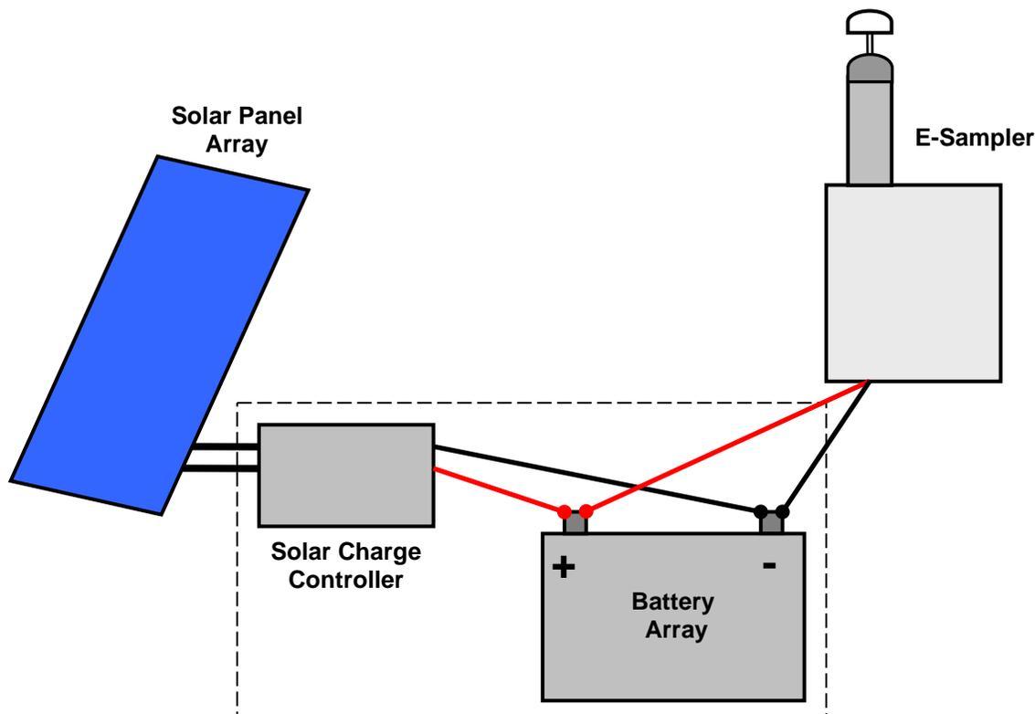
Figure 2-3 Simplified Solar System Diagram
