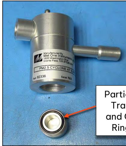
**Figure 8-1 Remove and Clean Particle Trap**
