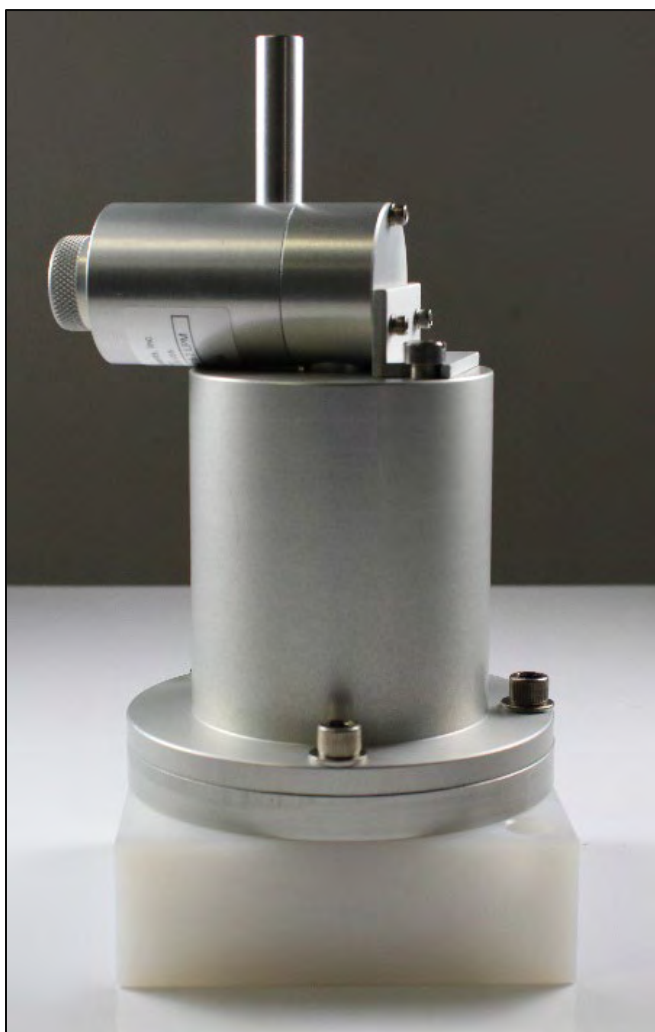
Figure 4-7 Sharp-Cut Cyclone and Canister Provides PM cut point, inverted canister within canister assembly block.
