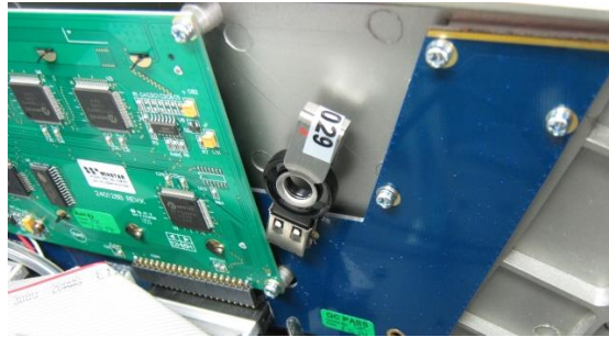
Figure 36 – Installation of USB Memory Stick
