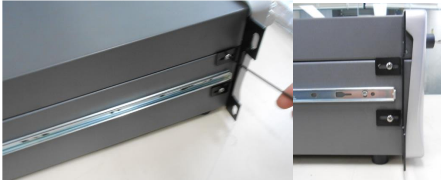
Figure 151 – Rack Mount Ears Fitted to Instrument
