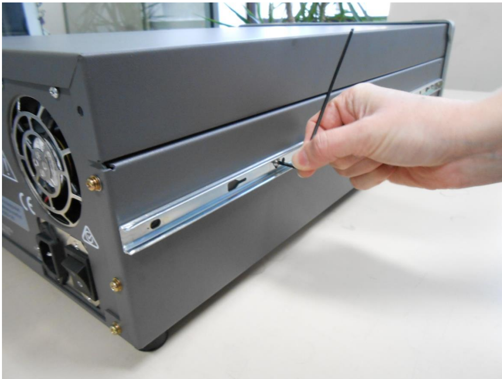
Figure 150 – Assemble Inner Slide on Chassis
