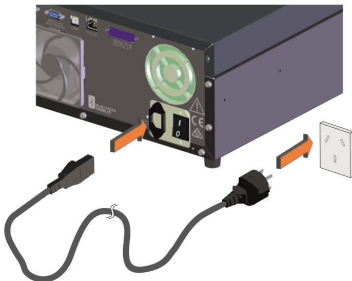
Figure 28 – Connect Power Cord
