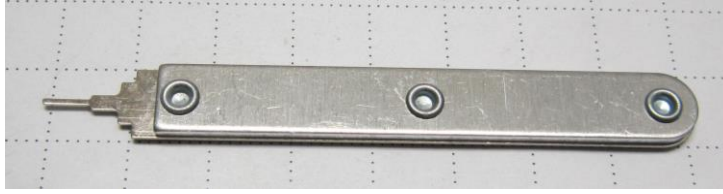
Figure 123 – Minifit Extraction Tool – (PN: T030001)
