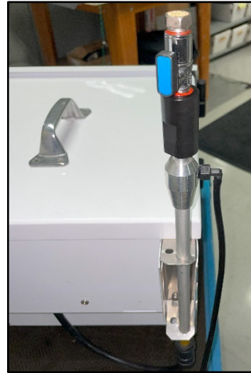
Figure 2-5 BC 1060 Inlet Location with Dilution Flow Adaptor
