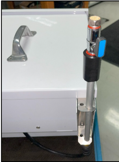
Figure 2-4 BC 1060 Inlet Location
