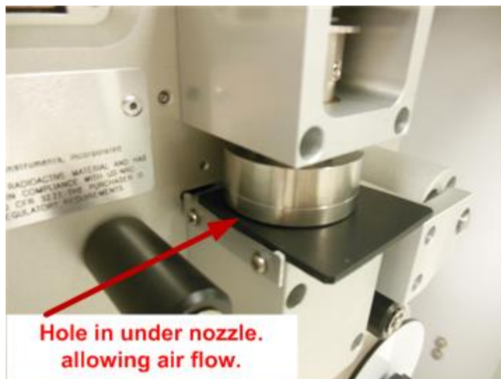
Figure 5-5 Nozzle Sealing Tool Upper System Test Configuration
