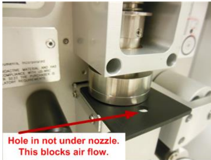
Figure 5-4 Nozzle Sealing Tool Lower System Test Configuration
