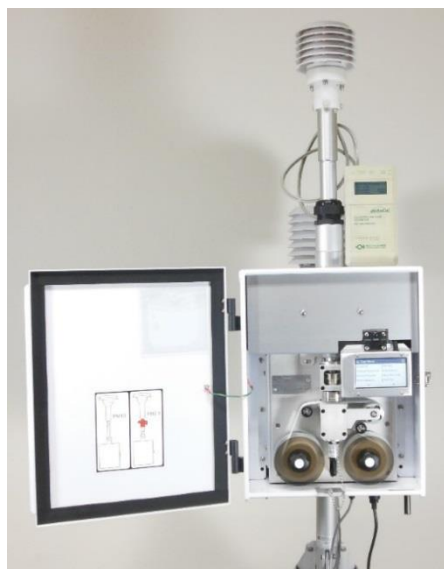
Figure 5-9 E-BAM with CTS Installed
