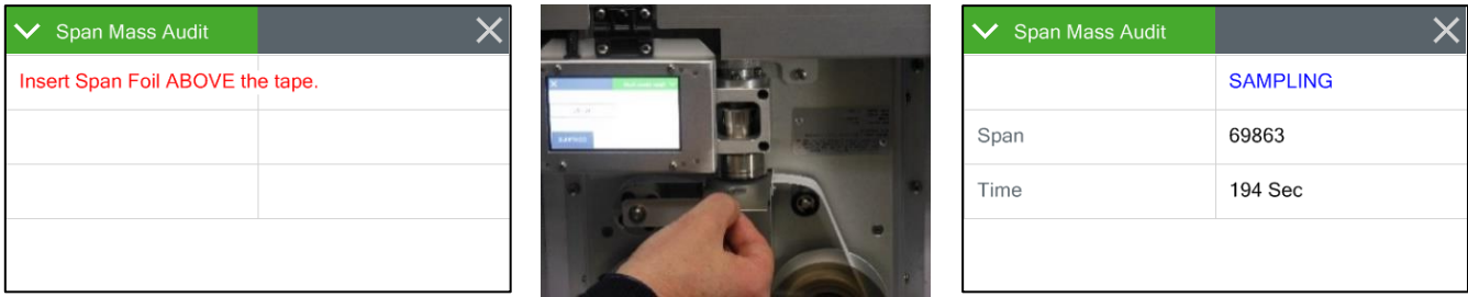
Figure 5-13 Starting the Span Test
