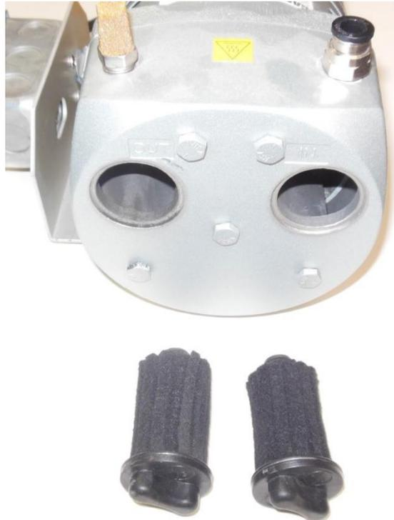
2. Remove the filter end caps from the front of the pump by unthreading the filter housings. Set these aside.
