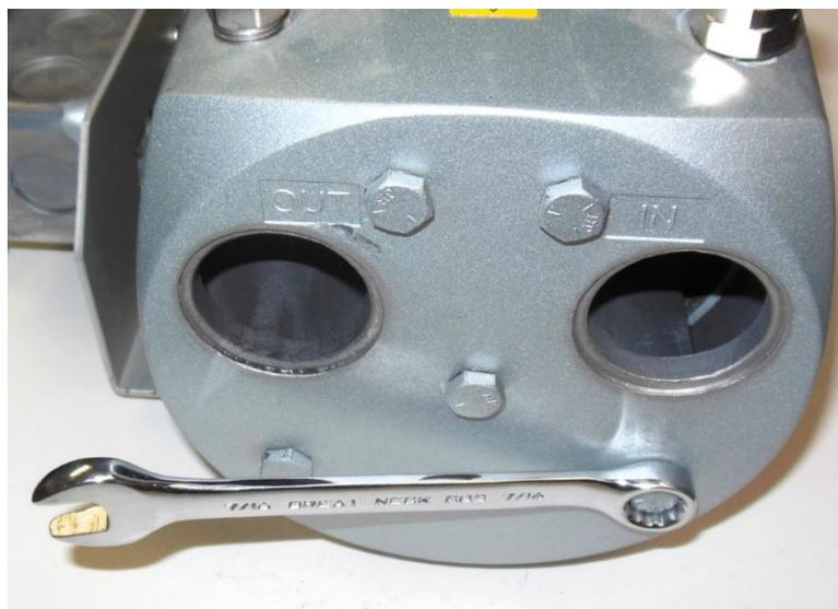
3. Remove the (5) muffer box bolts using a 7/16" combination wrench or socket wrench.
