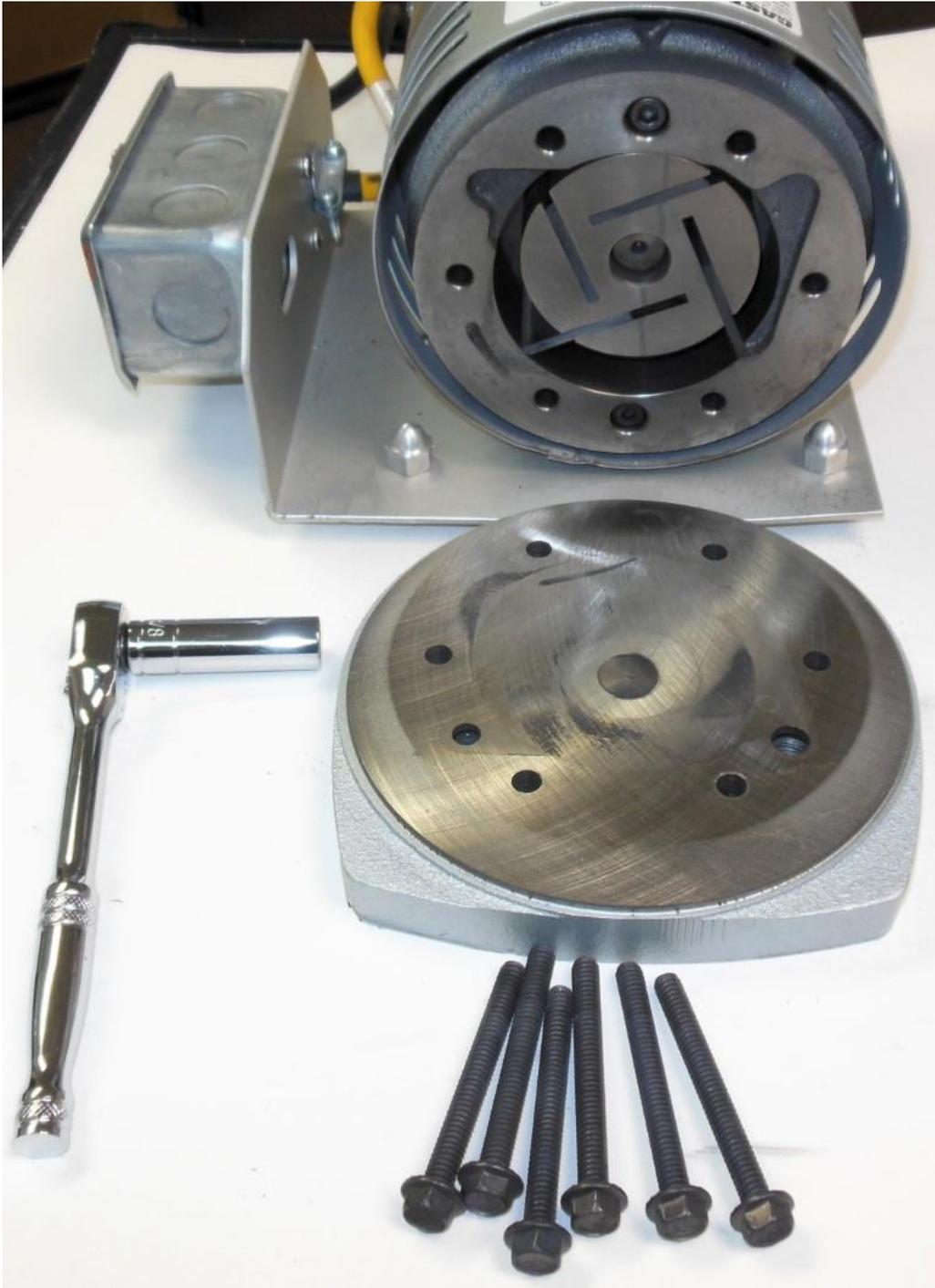
5. Using a 3/8" socket wrench, remove the (6) end plate bolts and remove the end plate.
