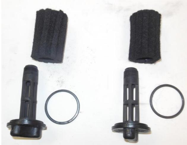
14. With the end caps removed, remove the filter and O-rings and replace them with the new units from the rebuild kit.
