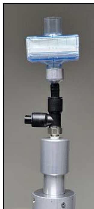
Figure 7-20 SigmaDust Adapter Installed on the Sample Conditioner
