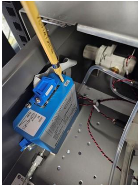
Figure 176 – Zero Flow Potentiometer Adjustment
