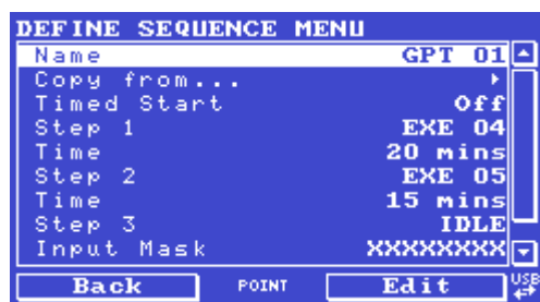
Figure 58 – Titration Sequence Setup
