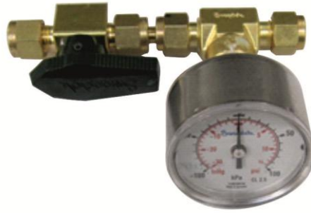
Figure 160 – Leak Test Jig - (PN: H050069)
