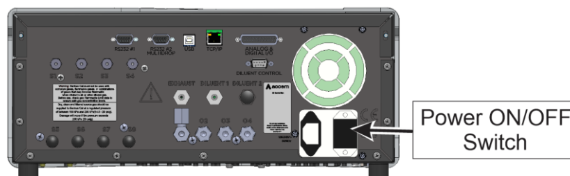
Figure 6 – Power ON/OFF Switch
