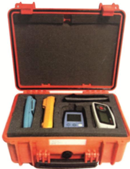
Figure 161 – Air Monitoring Test Equipment Kit (AMTEK) - Customisable
