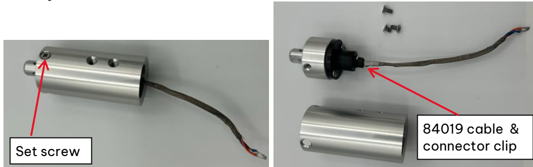
Figure 5-11 Accessing the 84019 Harness
