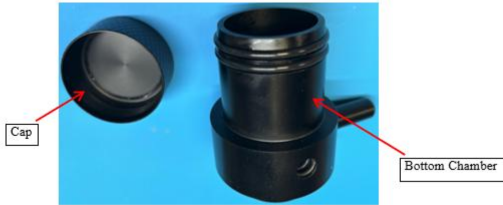
Figure 6-3 Lower Chamber and Cap
