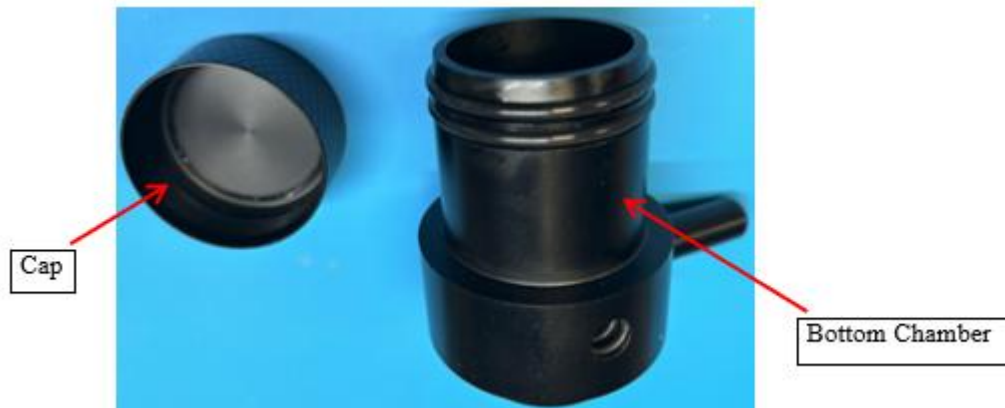
Figure 6-18 Lower Chamber and Cap Cleaning
