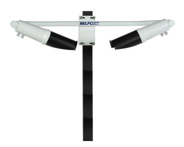
of background noise and natural variations in background light intensity. The sensors can asynchronously stream RS232 visibility data at user configured intervals, or can be operated in the polled mode, outputting information only when asked. Visibility is also compared to the preset relay thresholds, so that when an alarm condition is reached, the relay output is switched. Visibility thresholds can be set to any value within the instrument range.
